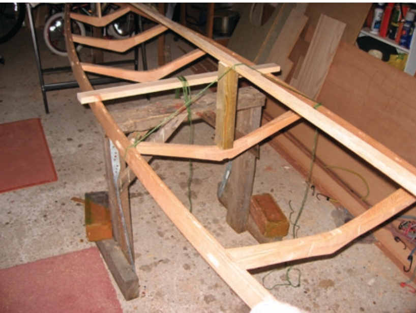
Deck structure strapped down onto a weighted trestle to achieve reverse sheer. Keelson in place. Photo Bill Samson
