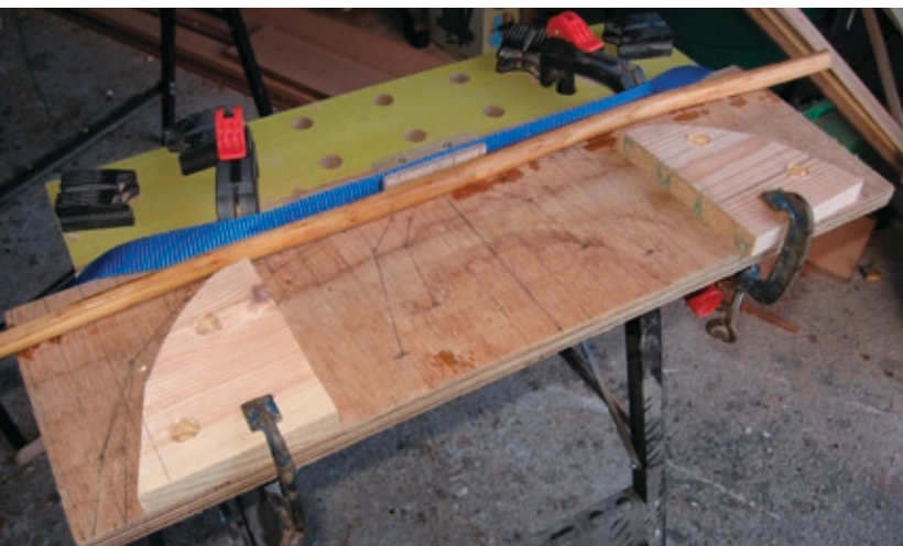
Rib bending jig with shapes at various stations marked on the surface. Photo Bill Samson
