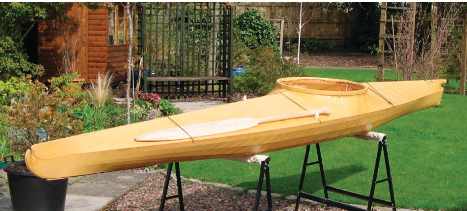
Frame skinned in loomstate cotton duck and waterproofed with linseed-oil varnish. Photo Bill Samson
