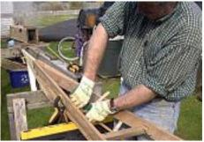
For pieces of wood I know to be difficult to bend I'll use an old rifle sling as a backing strip, an old leather belt would work as well.
