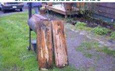
I built this box about 4 ft. long and about 6-inch square. I wanted something that I could steam four or five ribs at once. It needed less interior volume than the 8 ft. box I use for steaming coamings.
