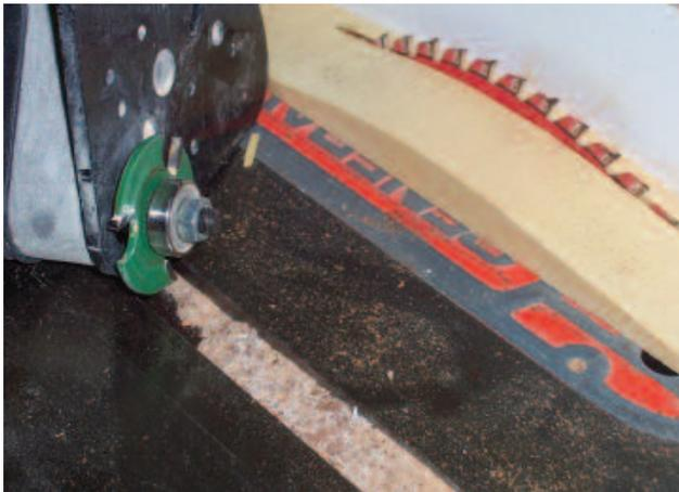
*The two options for ripping the spline groove are a router bit and a table saw blade through a shaped sub-table. Both cut  $\frac{1}{8}$ " wide and are set for  $\frac{1}{2}$ " depth of cut.*
