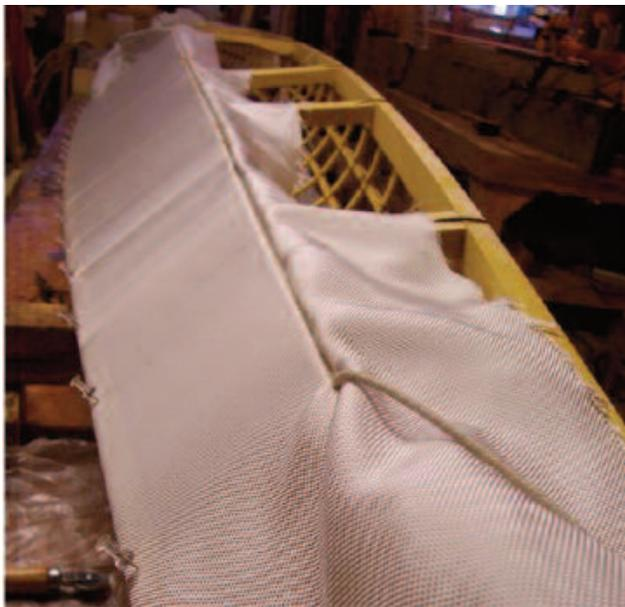
*Note the single spline groove down the center of the deck stringer*
