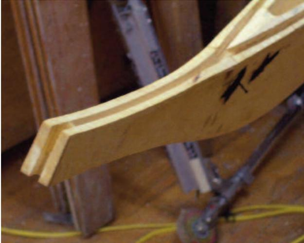
*Notice the smooth transition from two spline grooves to one. The groove wraps around the tip of the stem, but does not go any further.*
