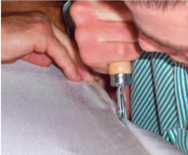
*An extra pair of hands help to tension and hold the skin as you roll the spline in. It is a good idea to wedge the spline just in the top of the groove along the whole boat before forcing it down to the bottom of the groove. This prevents large wrinkles from being formed as the skin is pulled into the groove.*
