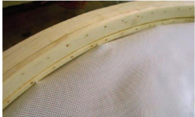
*Note the ends of the  $\frac{1}{8}$ " dowels, the  $\frac{3}{8}$ " lip separating the spline groove from the edge of the cockpit rim, and the spacing and locations of the tacks positioning the skin in preparation for trimming the fabric and inserting the spline.*
