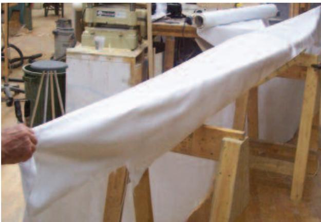
*Skin is stretched over the deck of the kayak first pulling out gross wrinkles and ensuring some degree of longitudinal tension in the skin.*
