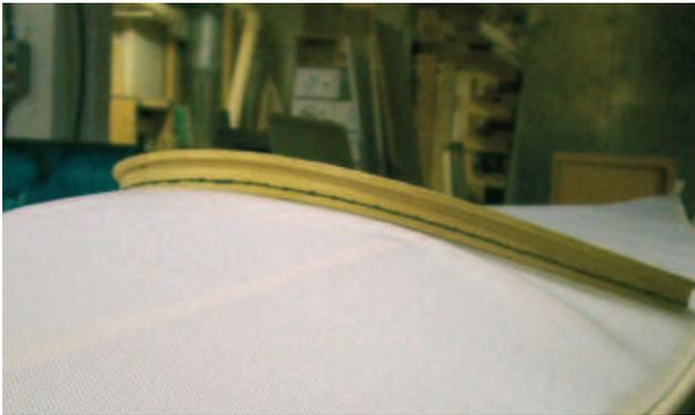
*Because a deck with no center seam has no slack skin to pull up into the rim, it needs to be sewn closer to the bottom of the rim. This means the stitches need to be spaced closer together.*
