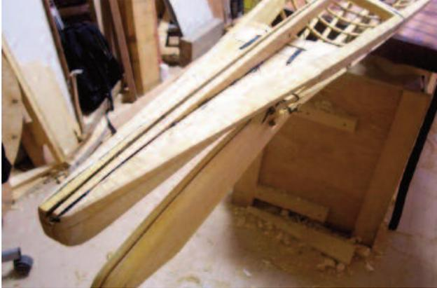
*The bow end of the bow deck stringer is rebated into the bow plate to enable it to feather out to flush at the tip of the bow, but still hold the splines and skin. I sewed the skin where the top and bottom meet.*
