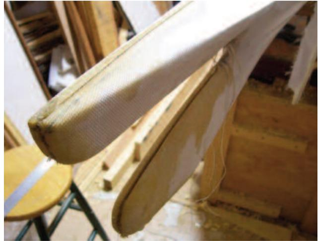
*Note the skin cannot be forced into the spline groove near the base of the jaw.*
