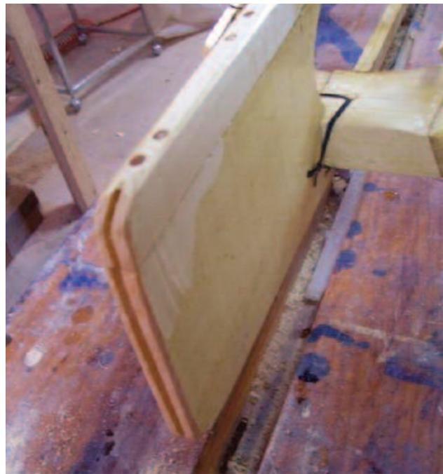
*The spline groove extends right to the bottom of the keel.*
