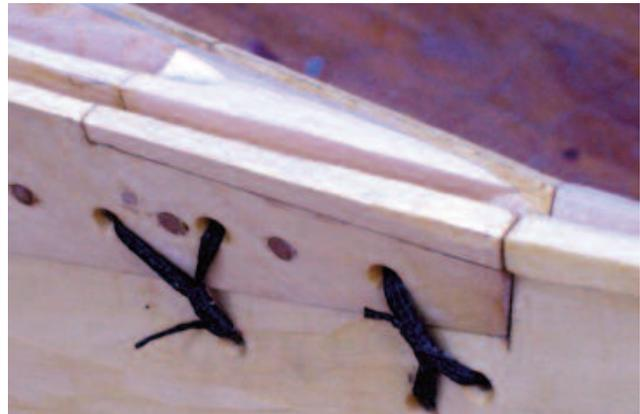
*Notice how the spline groove cuts the outside sections of the breast hook away. The only solutions are to avoid using a breast hook, use adhesive to hold the pieces to the gunwale, or double the thickness of the breast hook.*
