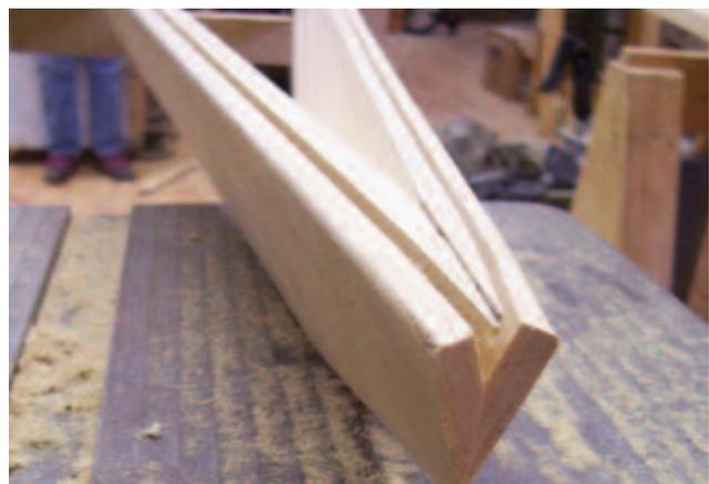
*The inside edges of the spline groove meet in a point and the outside dimension of the gunwale tips is the same as the stem material to be used, in this case just shy of  $\frac{3}{4}$ ".*
