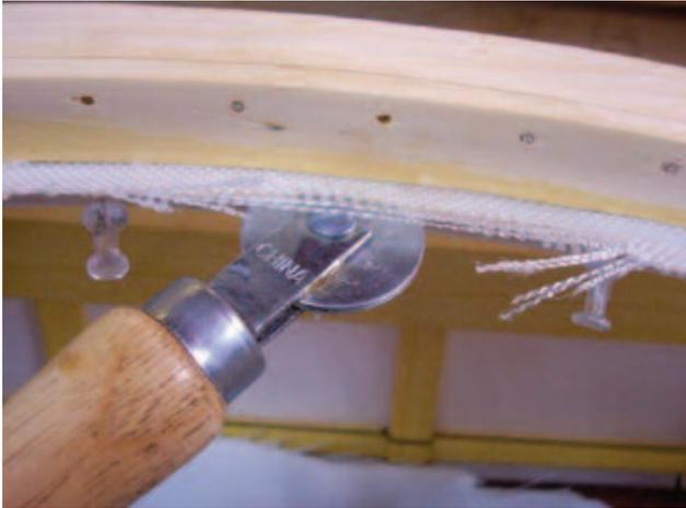
*Note how much of the fabric is pulled into the spline groove. The fabric was trimmed flush to the top of the rim. You can see how vulnerable the raw edge is to fraying. There is little margin for error. When in doubt, sear the edge!*
