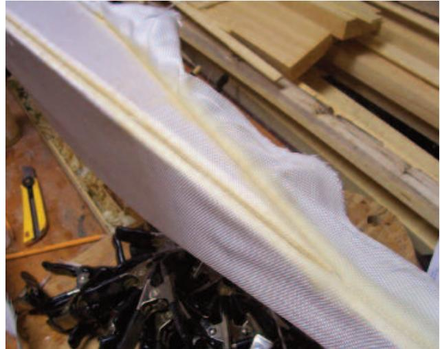
(21) Proceed around the front of the stem. I've found that a piece of scrap wood or steel a bit thinner than  $\frac{1}{8}$ " makes a good caulking iron to hammer the last little bit of cord over skin into the groove. Many layers of adhesive will seal the exposed cord, but it should sit slightly below the surface of the stem. If it does not, open the skin up and deepen the groove slightly with a hand saw.
